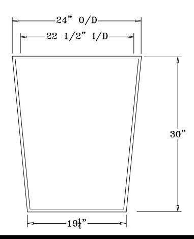
Top Diameter is 24". Middle diameter is 21". Bottom diameter is  $19\frac{1}{4}$ "
